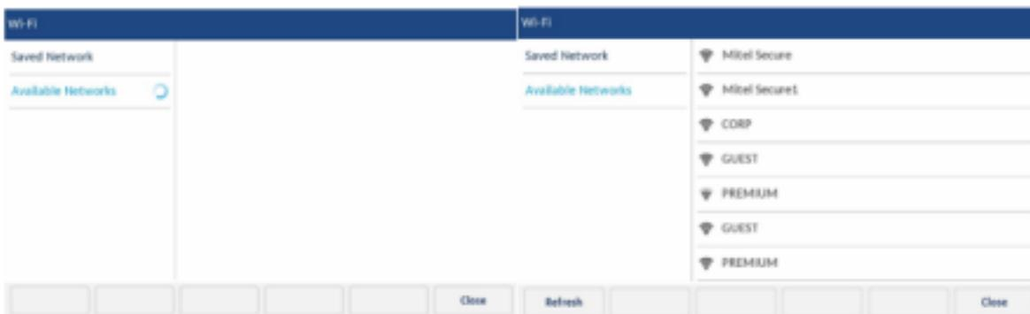
4. Select an SSID (that is, the name of a Wi-Fi network, for example, **Mitel Secure**) from **Available Networks** to connect. If the SSID is secured, a password prompt appears.
