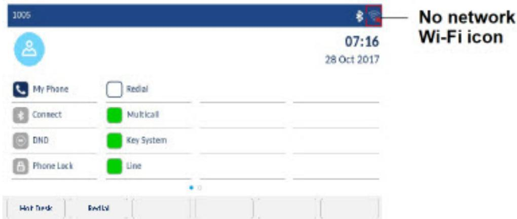
2. **Not Connected** - The phone is connected to the WLAN adapter but not connected to MiVoice Business or MiVoice Border Gateway.
