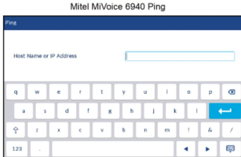
4. In the input field, enter the host name or IP address of the network endpoint you want to ping using the on-screen keyboard.
