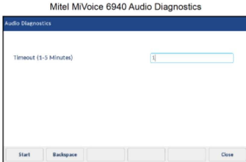
4. In the **Timeout** input field, enter the amount of time (in minutes from 1 to 5) you would like to run the audio diagnostic tool for using the dialpad keys.
